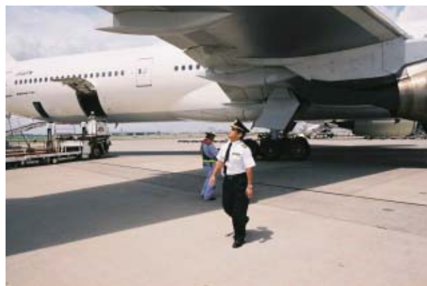
External visual inspection of fuselage and engine by flight crew
