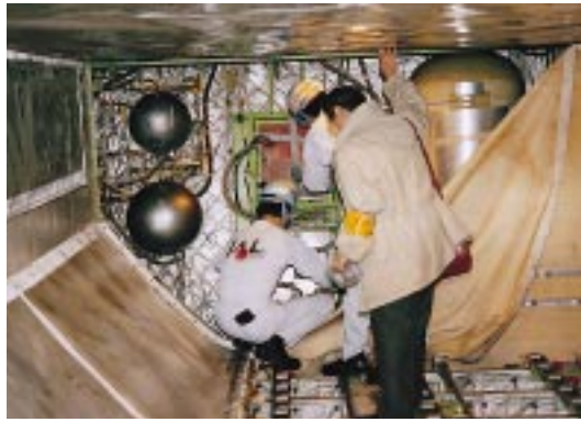
JAL aircraft are fitted with instruments for atmospheric measurement to help reduce pollutants.
