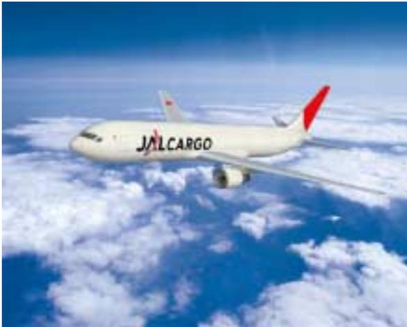
At its maximum payload of 60.5 tons, the 767 freighter has a range of 3,270 nautical miles (6,056 km). When carrying 50 tons the aircraft's range is 4,255 nautical miles (7,880 km).
