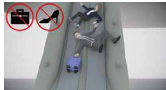
Slide damaged by baggage or high heels
