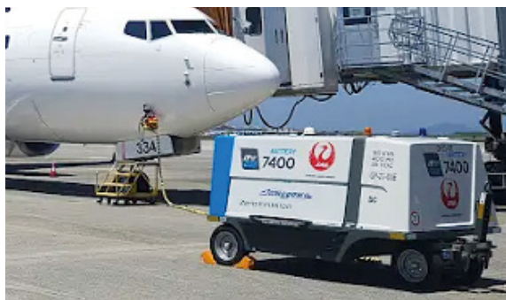
Lithium-ion-battery-powered Ground Power Unit (eGPU)
