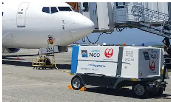
Lithium-ion-battery-powered Ground Power Unit (eGPU)
