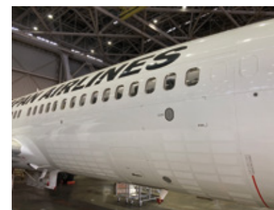
In November 2023, riblets were applied to a total area of approximately 25m 2 on the lower fuselage of a Boeing 737-800 aircraft.
