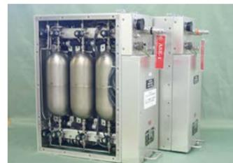
自動大気採取装置 (ASE: Automatic air Sampling Equipment)
