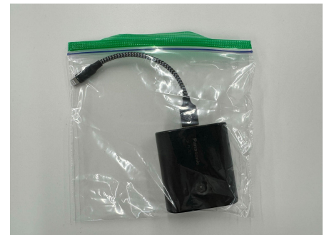
Example of short-circuit prevention for spare batteries
